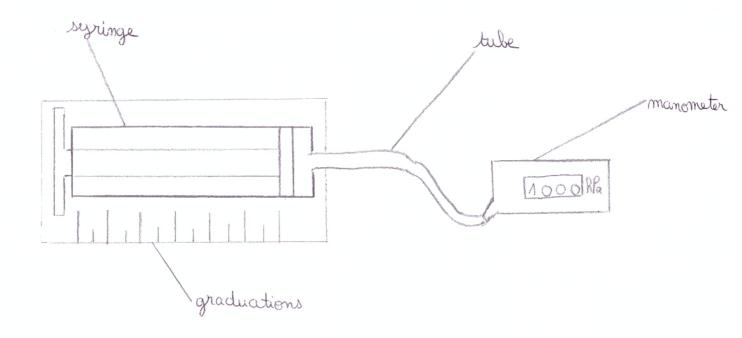
With this experiment we could demontrate the Boyle and Mariotte law. The result of the multiplication of the pressure and the volume is constant. So, when the pressure increases, the volume decreases.
