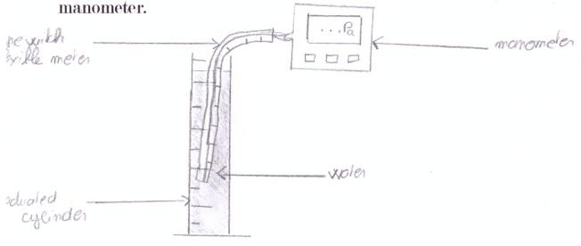
We measured the pressure at different depth and we made a graph. I we saw that the pressure accreased when the depth was bigger.
